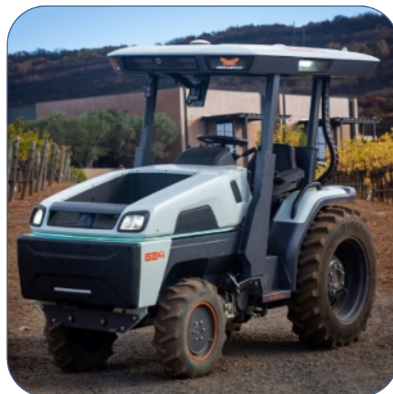
Figure 8 Monarch MK-V electric and fully autonomous tractor
